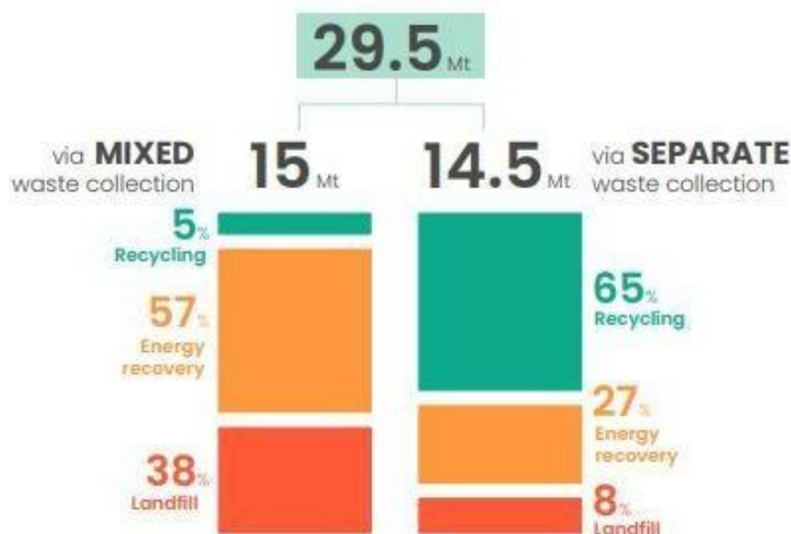
Figure 6 Differences between mixed and separately collected plastic waste in Europe. Source: Plastics Europe, 2022.
